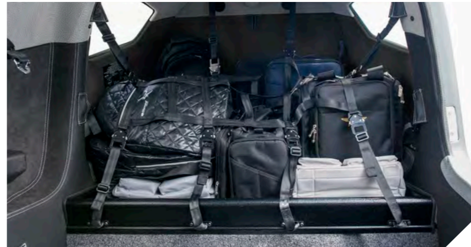
Rear baggage compartment in a 5-seat version: up to 120 kg / 265 lbs for your bags.
