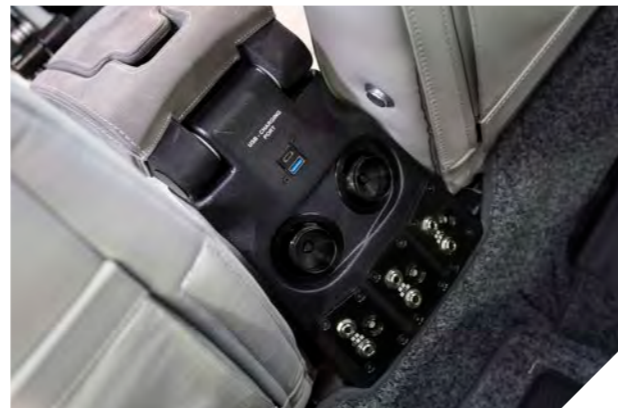
USB power outlets for pilot & co-pilot and passengers in the 2 nd row Dual headset plugs (LEMO connector + standard jack connector)
