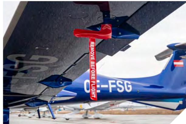
Heated pitot tube + pitot cover (Photo shows a DIAMOND MYO exterior design)
