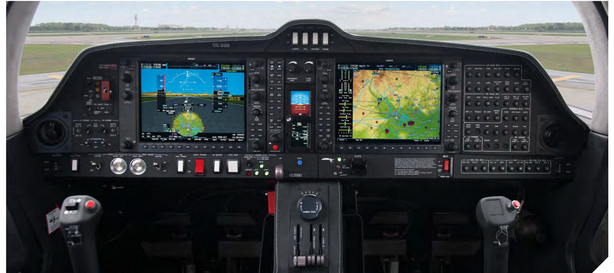
Integrated Garmin G1000 NXi glass panel cockpit
