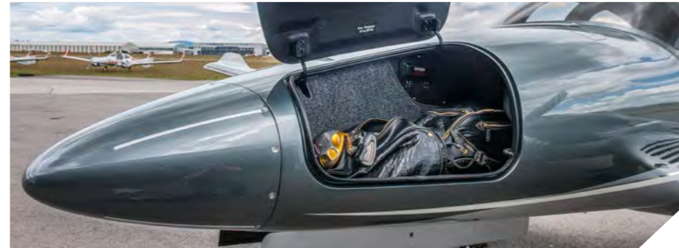
Front baggage compartment: up to 30 kg / 66 lbs for your personal belongings on each side. (Photo shows a DIAMOND MYO exterior design)
